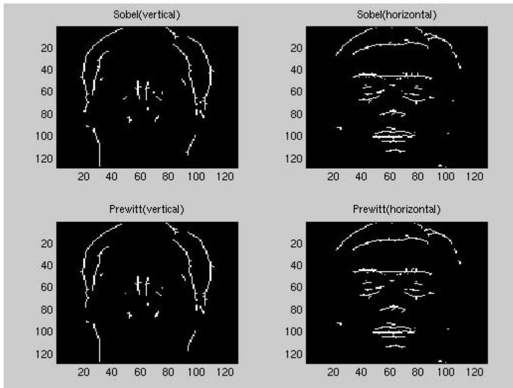
Figure 2: Detecting the edges of face a) Sobel-vertical b) Sobel horizontal c) Prewitt-vertical d) Prewitt-horizontal
