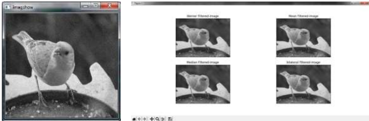
Figure 5: a) Image with Poisson Noise, density-80 and b) Weiner, Mean, Median and Bilateral filtered image
