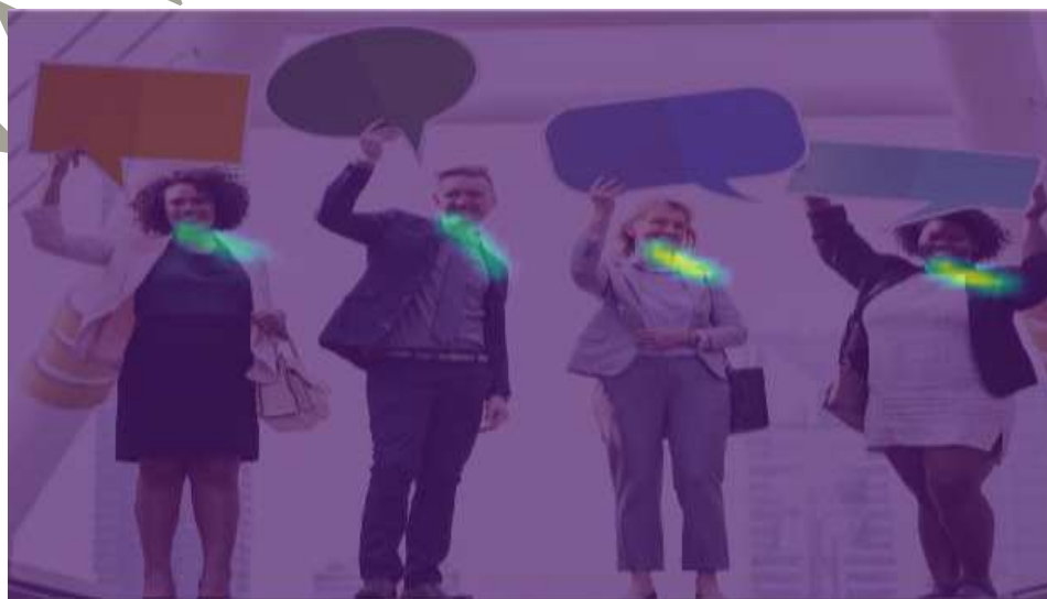
Fig 2: Showing Part Affinity maps for Neck – Left Shoulder pair for the given image
