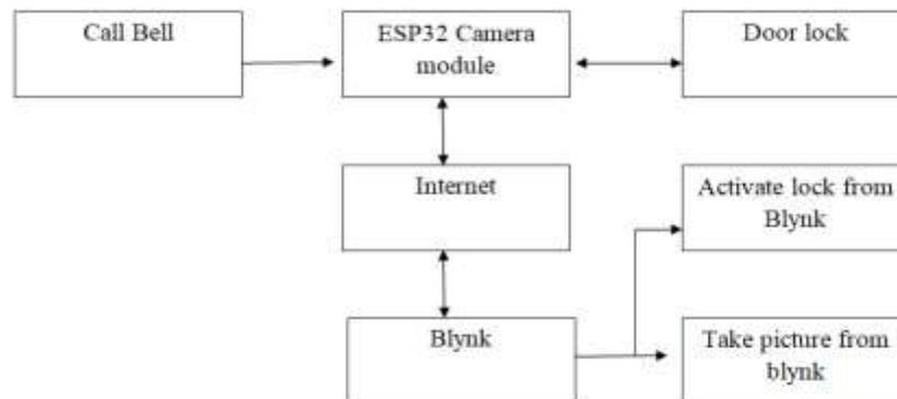
**Automation Process:** The above process is automated with the help of raspberry pi and face Recognition Technology. Once the Doorbell is pressed, camera module will get triggered and capture the image of the person. The input from the camera will be given to raspberry pi. The Raspberry pi is responsible for face Recognition and carry out further process. It will detect and recognize the faces using Haadcascade classifier and LBPH recognizer.
